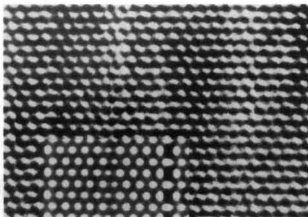
Fig. 13. High-resolution image of Matterhorn serpentine projected along the c axis together with the calculated image for underfocus 900 Å and thickness 86 Å.
