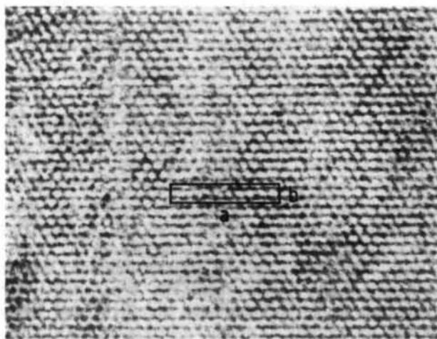
Fig. 6. High-resolution image of antigorite of Matterhorn surpentine projected along the c axis.
